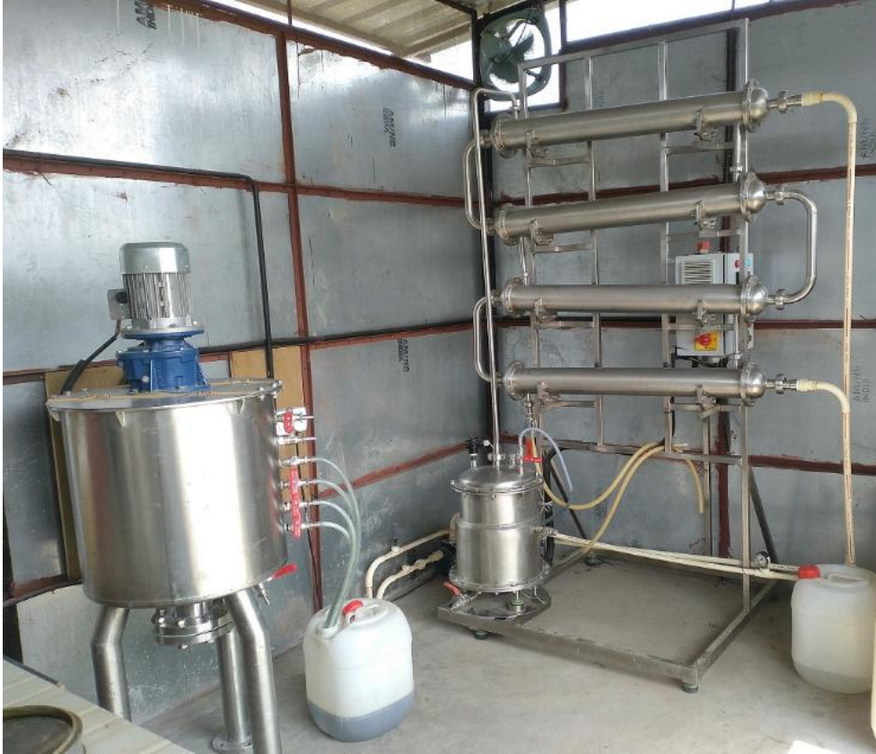
Pilot-scale wet algal lipid extraction system
